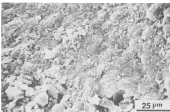
Figure 5 Debris on a mutually rubbed compressive fracture surface.
